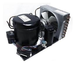
Figure 1. Condenser unit, model TCM2020E
