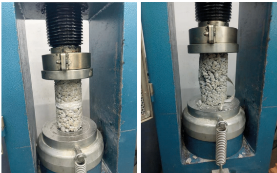
Figure 9: Axial compression strength test Elaborated by the author (2023) Figure 10: Rupture of the test specimen Elaborated by the author (2023)
