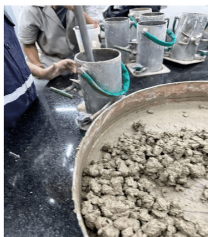
Figure 7: Concrete compaction Elaborated by the author (2023)
