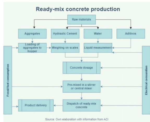
Figure 1. Typical Concrete Batching Process.
