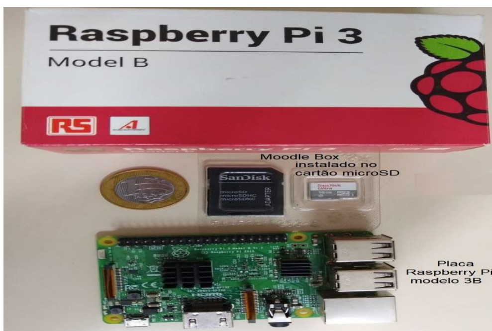
Figura 1- MoodleBox instalado no Raspberry Pi 3B
