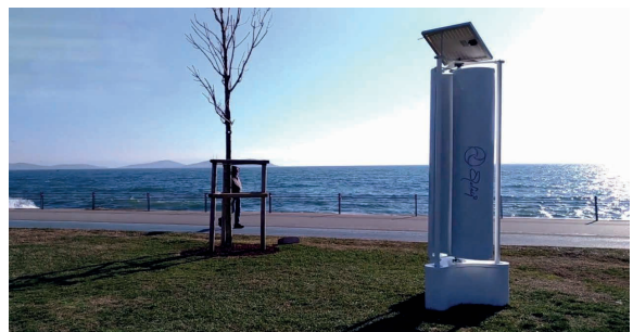
Figure 5 : Vertical Wind Power Generator in Liu
