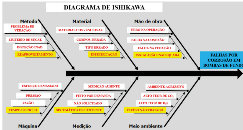
Figure 10 - Ishikawa diagram for corrosion pump failure.
