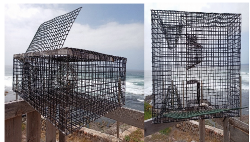
Figure 3. Rectangular trap design proposed for the experiment to capture P. platycerus .
