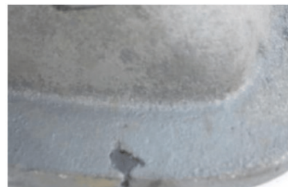
Fig. 5: Valve cover, showing an inclusion defect.
