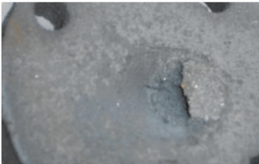
Fig. 3 shows a gray iron metallic piece with a shrinkage void at the center.
