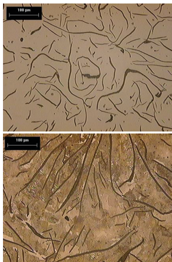
Fig. 1 and 2 show the microstructure of graphite distributed in a laminar form in gray iron at 100X magnification.
