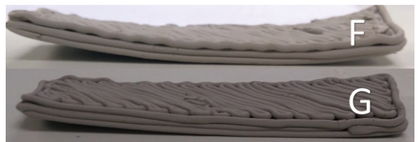
Figure 10: Warping of 3D Test Samples
