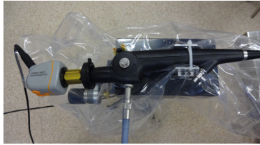
fig. 4: ureteroscope, endoscope camera and light cable coupling in the universal platform
