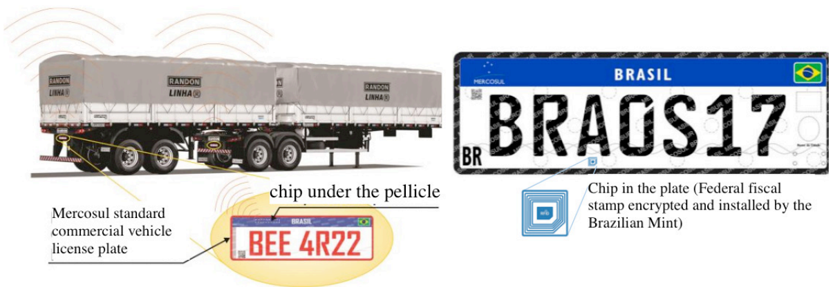
Figura 3: Automatic identification of road implements and SINIAV with a chip on the new vehicle identification plate (Barbosa, 2018).
