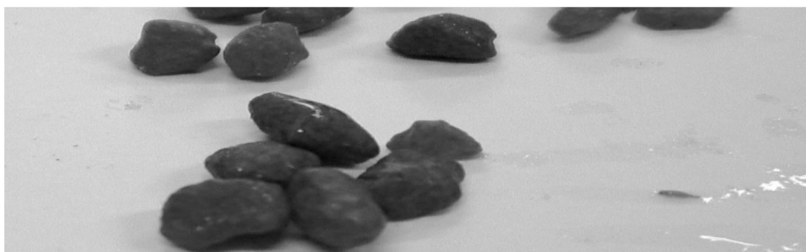
Figure 3: Example of fertilizer samples at the end of the experiment, after KCl release (thicker coatings – 8.45% and 9.30%)
