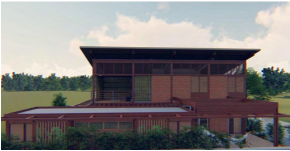
Image 12: East elevation view. Location of habitable platform and rooms. Opening for reception of winds.
