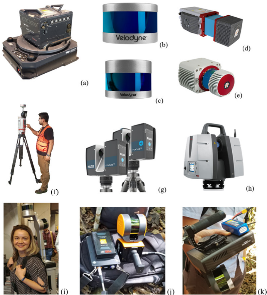
Figura 4. Exemplos de sensores TLS fixos e portáteis. (a) Teledyne Optech ALTM™ Galaxy; (b) Velodyne's Puck LiDAR sensor VLP-16; (c) Velodyne's Ultra Puck; (d) RIEGL VUX-1UAV; (e) RIEGL miniVUX-3UAV; (f) Riegl VZ-400i; (g) FARO Focus Laser Scanner 350; (h) Leica ScanStation P50; (i) LiBackpack D50 com dois sensores Velodyne VLP-16; (j) Laser scanner portátil ZEB Horizon; (k) Laser scanner portátil HOVERMAP™.
