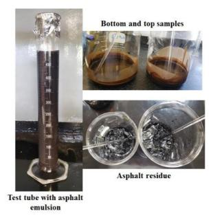
Fig. 5. Test of storage stability at 5 days.
