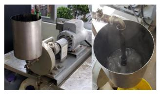
Fig. 1 Colloid mill used to reduce asphalt particle size and emulsify it.
