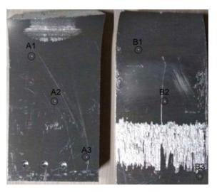
Figure 15 - Hardness Measurement Points/
