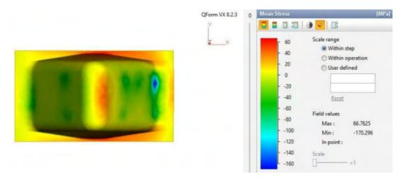
Figure 4 - Main Stresses in the Lower Matrix.
