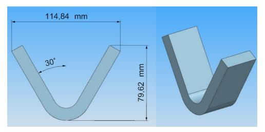
Figure 3 - Specimen After Deformation.
