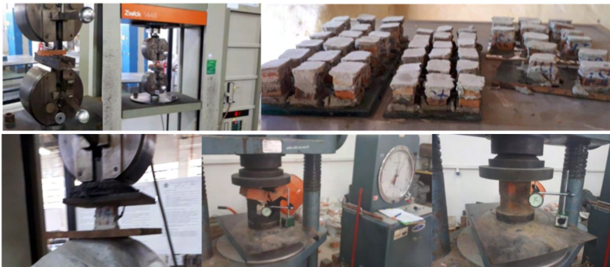
Photos 7 to 12: Bending tests, test pieces of bricks in press of 10kN capacity and full-scale bricks for compression and their corresponding press tests with a scale of 10,000 kgf. (own elaboration, Plastic Technology Lab at FIUNA and Construction Materials Lab., FIUNA).
