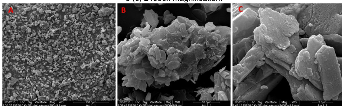
Figure 14 - SEM micrographs of the clay sample. (a) 800x magnification, (b) 6000x magnification e (c) 24000x magnification.
