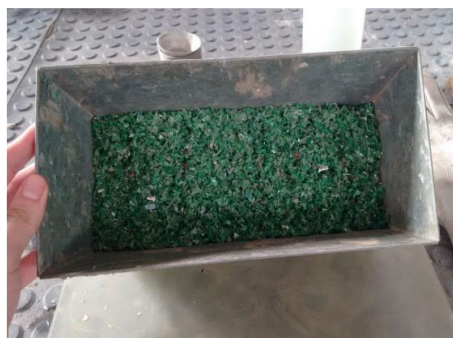
Figura 2. Material passante na peneira 4,8mm – PET.
