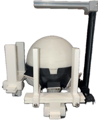
Fig. 8. Motion-tracking system 3D-printed structure.
